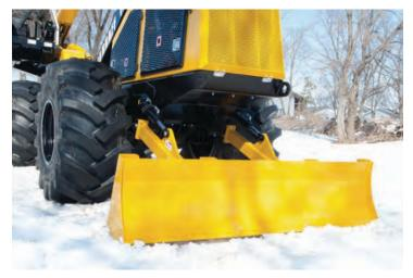
The Jarraff's **PUSH BLADE** features an improved approach angle and updated blade design for better field performance. Push button controls make brush clean-up fast and efficient.
