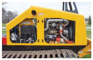
The **CUMMINS QSF 3.8L 130HP TIER 4 DIESEL ENGINE** meets all EPA regulations, while improving overall fuel efficiency and roading speed. The engine positioning allows for easy access and service.
