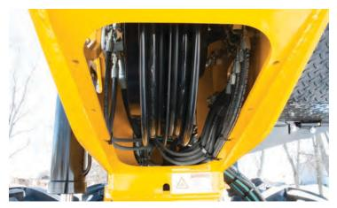
**INTERNALLY MOUNTED HOSE REEL** protects crucial hydraulic hoses from the elements and from any falling debris.
